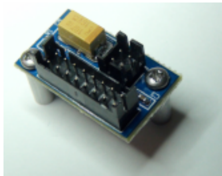
Figure 1 MK-24316 PIC16F1825 Based I2C Slave for PWM Servo Control or Ultra Sonic Sensors
