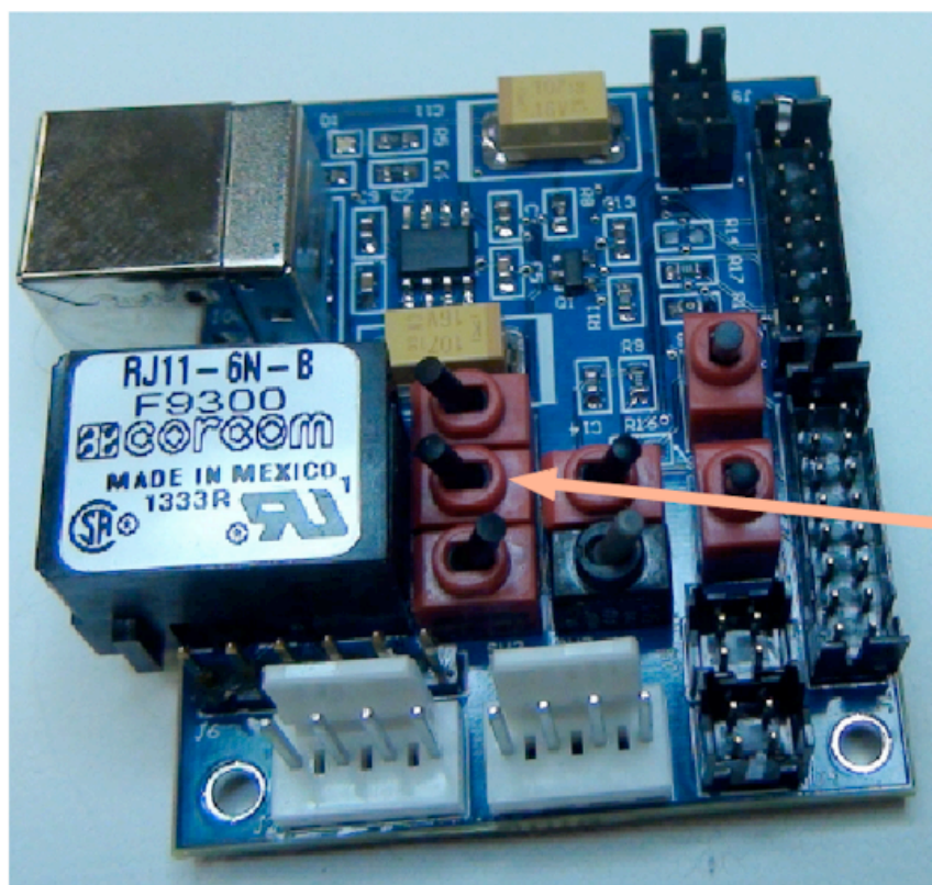
Figure 3 Switch 3 used to configure the I2C bus supply for 5V or 3.3V Operation.
